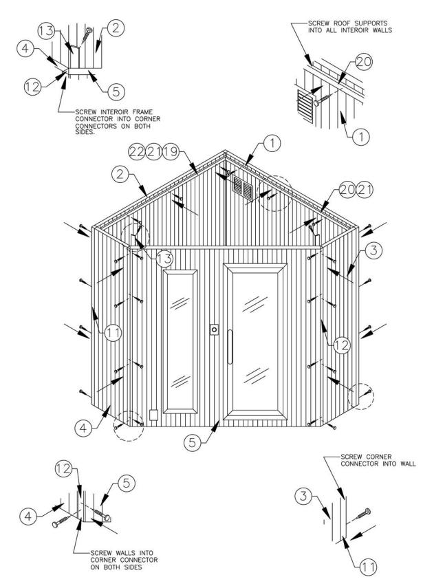
Figure 5. Attaching the front wall with door
